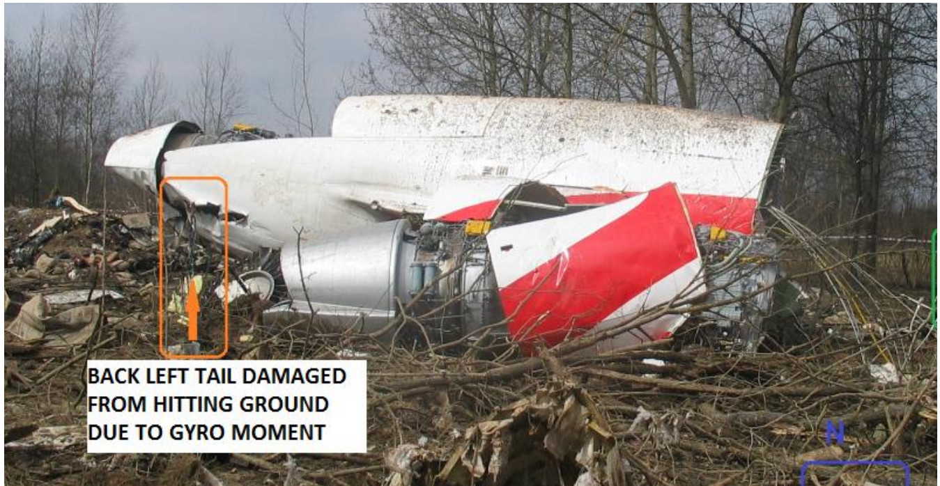
Fig. 20. The back part of the tail was damaged by the centre motors gyro moment when the right motor broke off.
