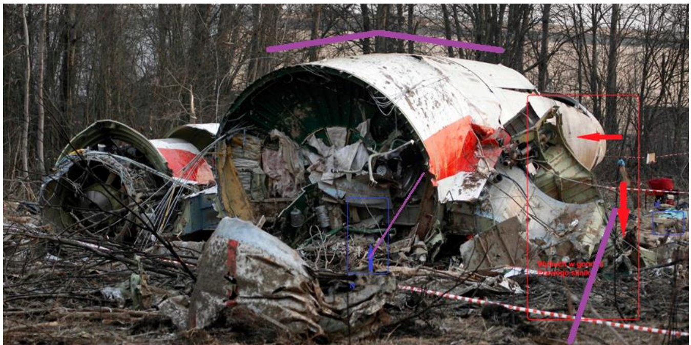
Fig. 21. The tail fuselage shows sign of the struggling between the gyro moments of the centre motor and right motor. Also notice the structure is twisted downwards inside the fuselage, indicating this structure was separated from the rest of the fuselage at the time of impact.
