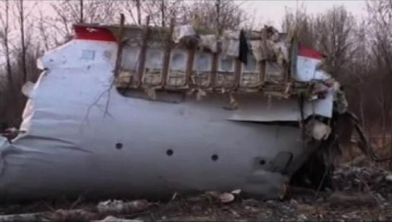
Fig. 9. The front bottom section below the president's salon. The entire top section is pulverized and the window section was thrown outwards most likely caused by the high internal pressure at the near ground explosion. Note the windows have not been in ground contact.
