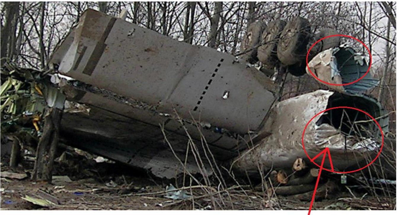
Fig. 10. The left wing root shortly after the crash. The portion shown in the pictures left side was originally facing towards the fuselage. Notice the wheels are soiled on the inwards side of both rows, but not along the entire rim, only at the small portion of the rim, that was facing downwards during the sideways sliding/turning movement of the wing piece. Also notice the end of the wheel house shows indication of being hit by an object (most likely a tree) from the wings topside during the roll movement described below
